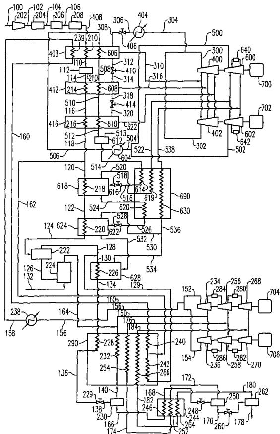
**(57) Abstract:** Natural gas liquefaction system employing electric motors as compressor drivers. A combination of motors and steam turbines can be powered by a cogeneration plant and employed as drivers.
