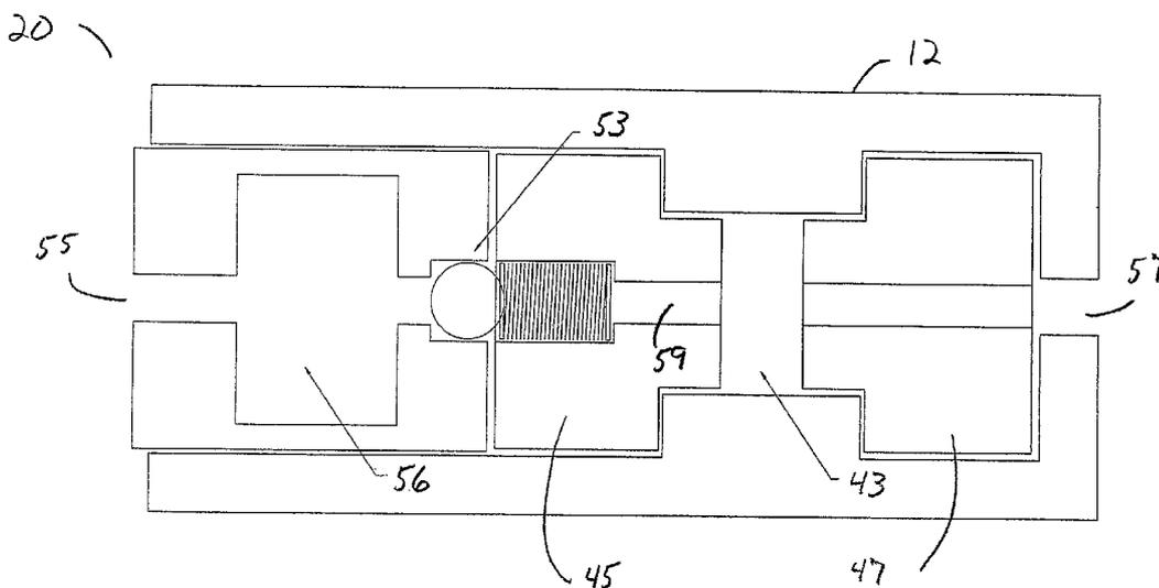
(57) Abstract: A liquefaction surgical handpiece having a capacitance chamber upstream of the boiling chamber.
