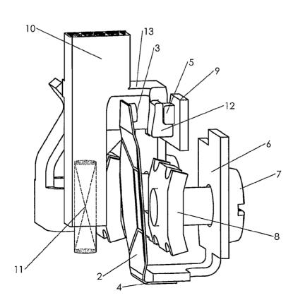
(57) Abstract: An electrical receptacle has an outlet and senses the operating temperature and automatically turns off when the temperature rises above a predetermined threshold. The receptacle has a reset button that must be manually operated to enable operation of the outlet to resume.
