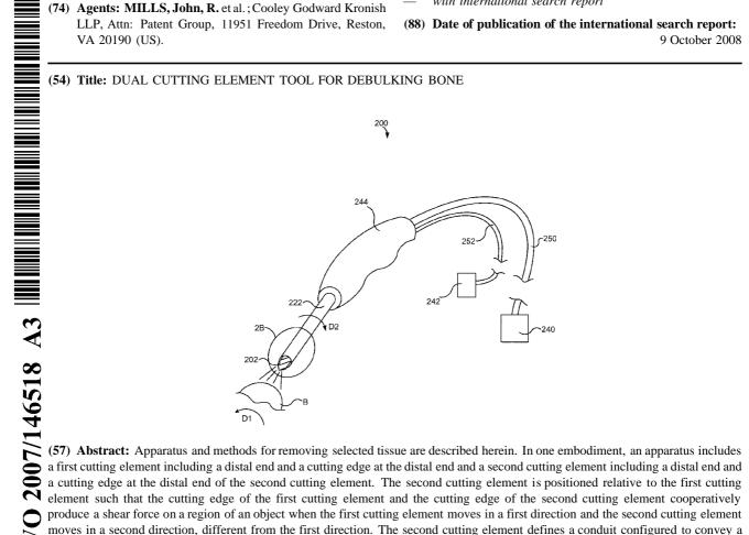
produce a shear force on a region of an object when the first cutting element moves in a first direction and the second cutting element moves in a second direction, different from the first direction. The second cutting element defines a conduit configured to convey a fluid from the region of the object.
