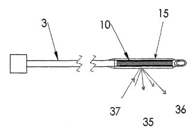
(57) Abstract: An echogenic surface surgical instrument, more particularly an echogenic surface surgical needle for use in ultrasonic imaging to facilitate real-time ultrasound imaging and monitoring of the needle during surgical procedures. At least a portion of a structural surface of the needle comprises grooves to entrap gas column.
