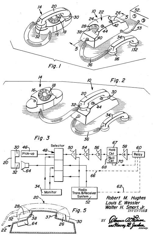
SWITCHING SYSTEM FOR RADIO-TELEPHONE SYSTEM
