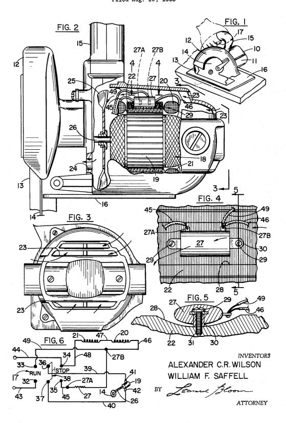
3,260,873 MOUNTING AND COOLING MEANS FOR AN ENERGY-DISSIPATING RESISTOR IN AN ELECTRICALLY-OPERATED DEVICE
