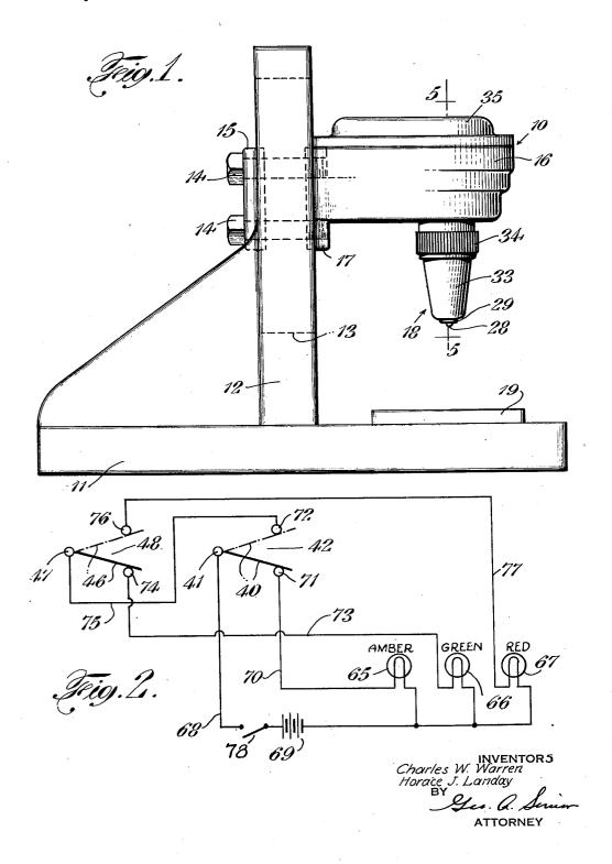
TOLERANCE-LIMIT COMPARATOR GAUGE
