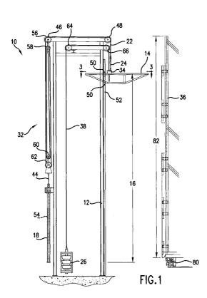
(57) Abstract: An elevating platform assembly is provided. In accordance with one exemplary embodiment a platform is present and is moveable along a travel distance of a mast. A cylinder is provided and is capable of being actuated. The cylinder is used to move the platform along the travel distance.
