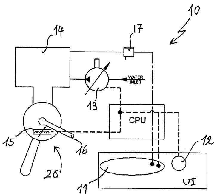
(57) Abstract: In an improved method and machine for espresso coffee there are provided one or more operating units (10) each of which comprises a boiler, a pump, a heating unit, a group (26) for aroma extraction and dispensing of the espresso coffee brew, including related conduits. Each unit (10) is equipped with a system for controlling and adjusting the espresso coffee brewing parameters, in particular the water pressure.
