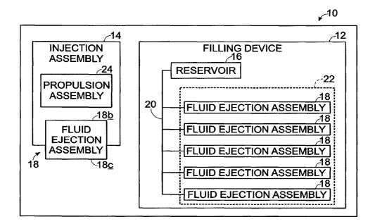
(57) Abstract: The present invention provides method and apparatus for providing high throughput injections. In one embodiment the invention provides a filling device adapted to deliver injectate from a common reservoir to a plurality of disposable fluid injection assemblies and a reusable propulsion assembly adapted to receive a filled disposable fluid injection assembly and deliver an injection to a patient.
