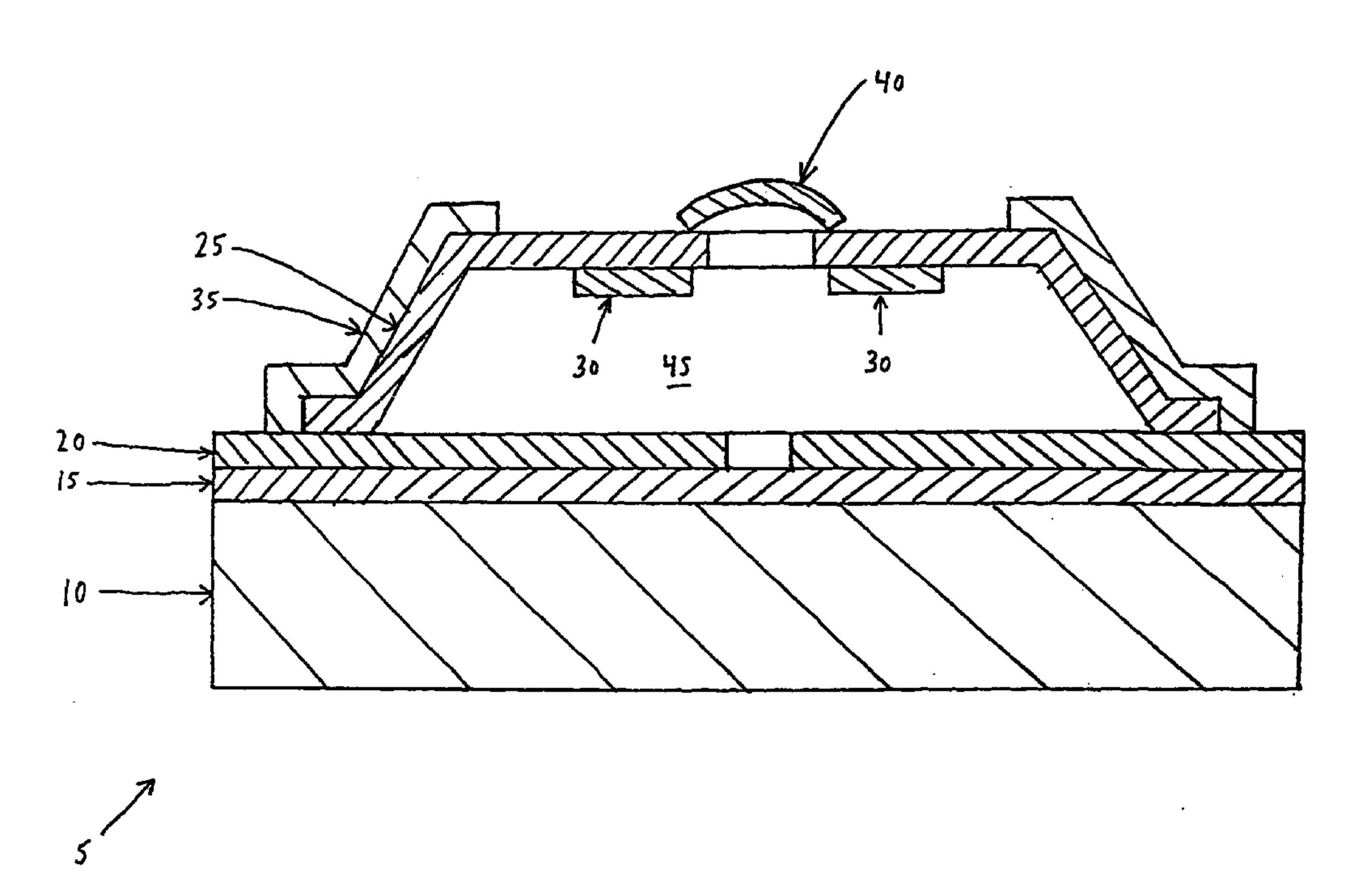
(57) Abstract: A tunable Fabry-Perot filter (5) and a tunable vertical vacity surface emitting laser (VCSEL) (5) are disclosed, where both devices utilize an improved dome structure (40) for creating an internal air gap.
