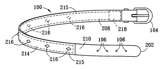
(57) Abstract: A collar (100) to which is mounted an illumination source (218) and one or more insets (216). Each of one or more light-transferring fibers (302) includes a first end (302a) coupled for receiving light from the illumination source (218), and a second end (302b) coupled for transmitting light to an inset (216).
