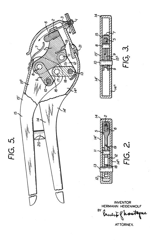
3,048,296 AND-OPERATED TOOL FOR RIVETING BY MEANS OF TUBULAR RIVETS RECEIVING A HAND-OPERATED SHANK
