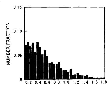
GRAIN SIZE OF RETAINED AUSTENITE GRAIN ( $\mu m$ )
