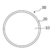
When the Cu alloy core material further contains one or more of Ni, Zn, Rh, In, Ir, Pt, Ga and Ge in an amount, for each, of 0.011 to 1.2% by mass, it is able to increase the reliability of a ball bonded part in a high-temperature environment of 170° C. or more. When an alloy skin layer containing Au and Pd is further formed on a surface of the Pd coating layer, wedge bondability improves.
