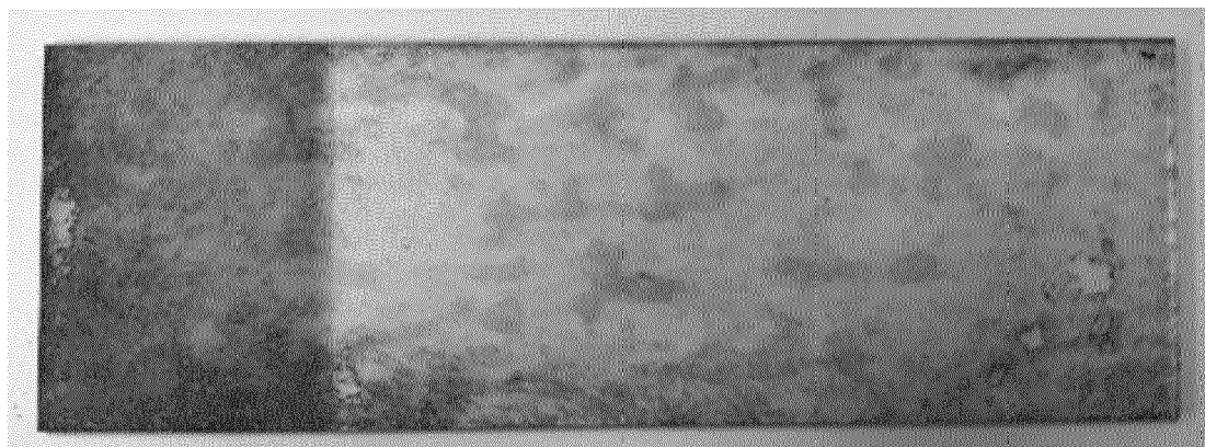
Glass substrate coated with Ketjen black
