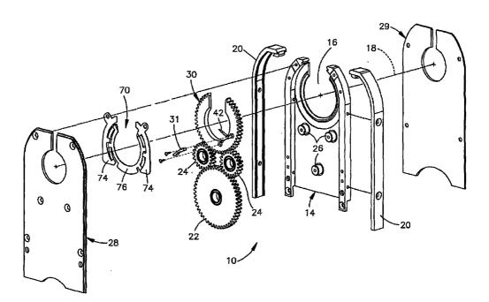
(57) Abstract: An orbital weld head includes a metal insert and rotor. The covers are made from mica laminate. A metal spring/brush that is preferably one piece side loads the rotor against the insert. The rotor and insert have interengaging portions, preferably trapezoidal, that cause the rotor to move axially when it expands from heat, thus minimizing binding.
