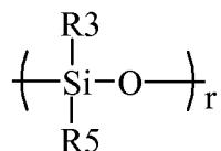
15 where  $\text{R}_3$  and  $\text{R}_5$  are as previously defined and where  $r$  is an integer of 3 to 7. Preferred are the cyclic siloxanes where  $r$  is 3 or 4 and  $\text{R}_3$  and  $\text{R}_5$  are both methyl, these cyclic siloxanes being hereafter designated  $D_3$  and  $D_4$ , respectively.  $D_3$ , which is a strained ring structure, is especially preferred.
