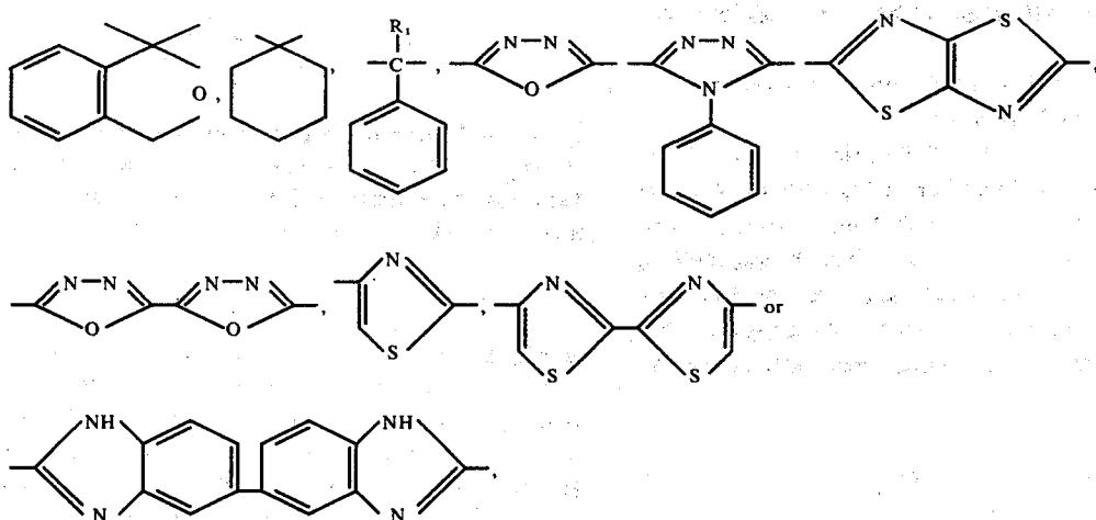
wherein  $R_1$  represents a hydrogen atom, an alkyl radical having from 1 to 4 carbon atoms, a phenyl or a cyclohexyl radical, and  $X$  represents an alkylene radical having less than 13 carbon atoms. The various phenylene or cyclohexylene radicals can be substituted by methyl groups.
