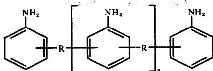
wherein  $y$  represents a number from 0.1 to about 2, R represents a divalent hydrocarbon radical having from 1 to 8 carbon atoms derived from an aldehyde or ke-
