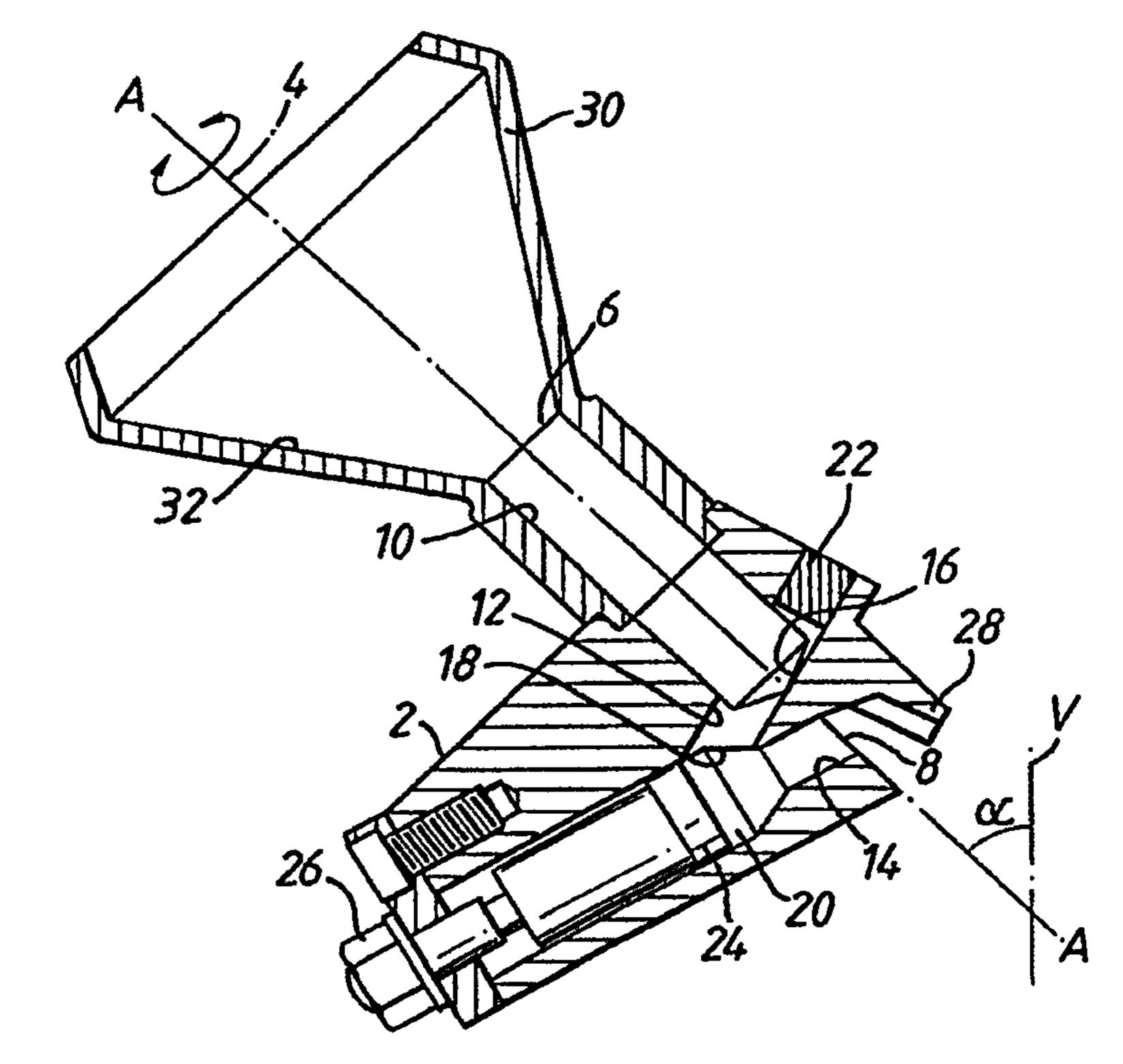
volume of particulate substance, so as on rotation to provide movement of the contained particulate substance at the inlet (6) and thereby ensure the flow of particulate substance to the metering chamber (20).
