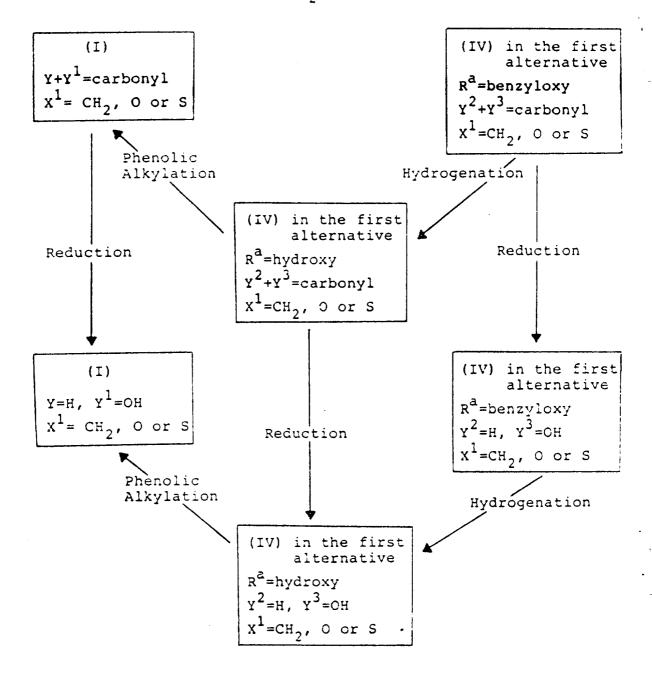
The reaction is generally carried out in a reaction-inert solvent, lower alcohols such as methanol being particularly well suited for this purpose. The temperature conditions for this transformation are not critical, e.g., 0-70° C. is generally satisfactory, with ambient temperature particularly well suited as a matter of convenience.
