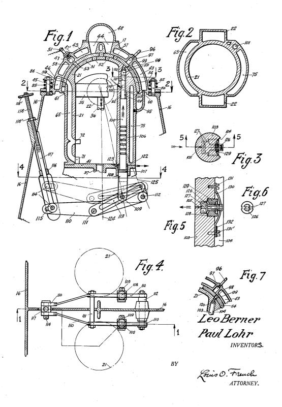
FUEL INJECTION APPARATUS FOR INTERNAL COMBUSTION ENGINES
