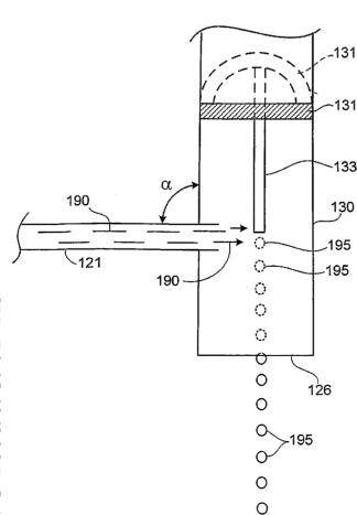
(57) Abstract: Particles and related methods are disclosed. In some embodiments, a method of making particles can include forming a stream of a mixture including first and second materials, exposing the stream to a vibration, and treating the stream to form particles. The vibration can have, for example, a sinusoidal, triangular, and/or sawtooth waveform.
