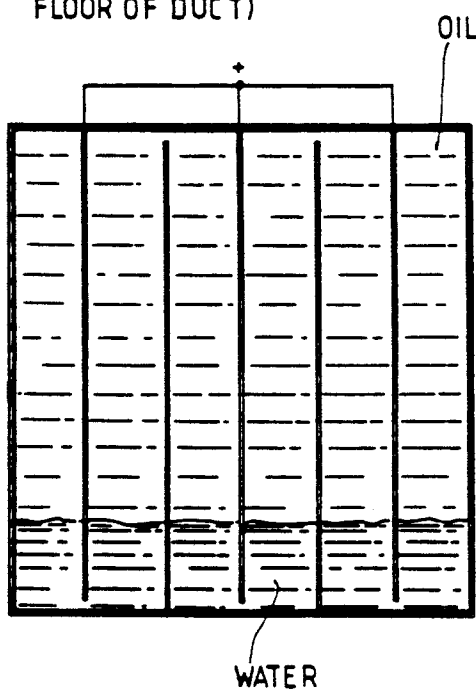
FIG.2D (WATER SEGREGATED AT FLOOR OF DUCT)
