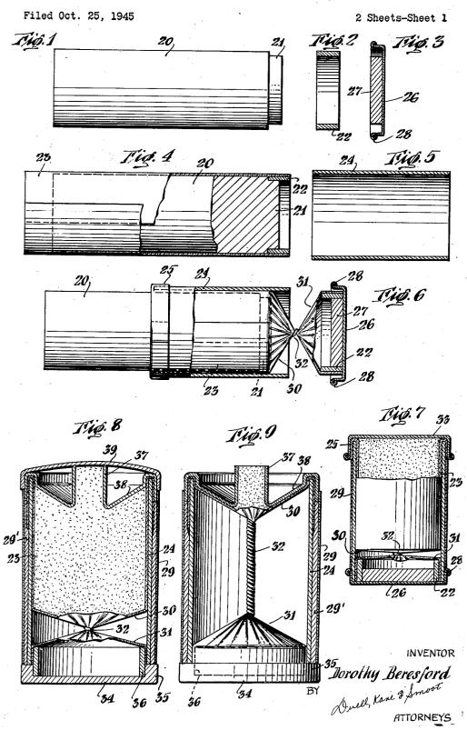
TWISTING TYPE COLLAPSIBLE TUBE DISPENSER
