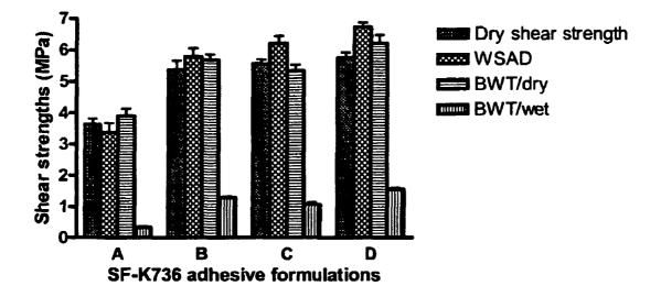
SF-K736 adhesive formulation: the total solids content, 50%; SF:K736 weight ratio, 10:1; **A**: SF only; **B**: SF + K736; **C**: SF + K736 + NaOH (NaOH, 1 wt%); **D**: SF + K736 + Na<sub>2</sub>B<sub>4</sub>O<sub>7</sub> (Na<sub>2</sub>B<sub>4</sub>O<sub>7</sub>, 0.69 wt%); The weight precentages of NaOH and Na<sub>2</sub>B<sub>4</sub>O<sub>7</sub> were based on the total solids content.
