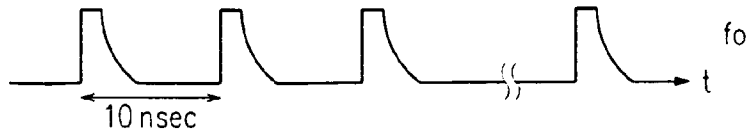
Fig. 7A VOLTAGE SIGNAL AT TARGET MEASUREMENT PORTION
