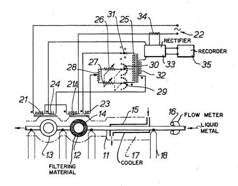
3,387,209 METHOD AND APPARATUS FOR MEASURING THE METAL OXIDE CONTENT OF LIQUID METAL
