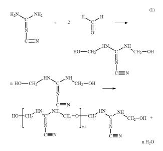
**[0117]** Thus, the molar ratio of formaldehyde to dicyandiamide is preferably located within the range from 0.8:1 to 4:1, in particular from 1:1 to 3:1. A molar excess greater than 4 does not provide any additional advantage but may result in an undesirable general setting.
