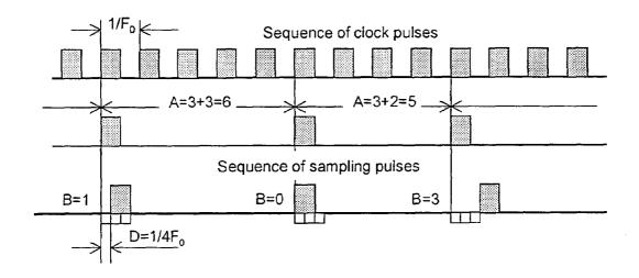
FIG.3. A time diagram showing the manner in which the sampling pulses are formed
