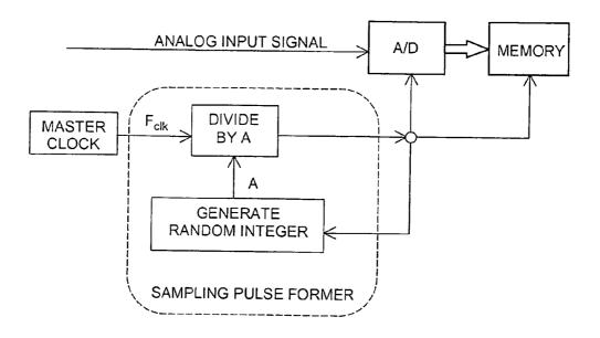
FIG. 2. A schematic block diagram of a priori art circuit
