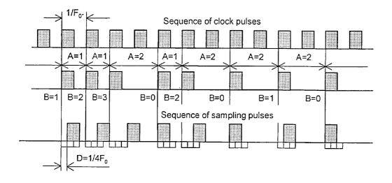
FIG.4. A time diagram showing the manner in which the sapling pulse sequence is adapted to the highest rate operation
