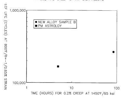
(57) Abstract: A nickel based superalloy composition comprising 16.0 to 20.0 weight % Co, 9.5 to 11.5 weight % Cr, 1.8 to 3.0 weight % Mo, 4.3 to 6.0 weight % W, 3.0 to 4.2 weight % Al, 3.0 to 4.4 weight % Ti, 1.0 to 2.0 weight % Ta, 0.5 to 1.5 weight % Nb, 0.01 to 0.05 weight % C, 0.01 to 0.04 weight % B, and 0.04 to 0.15 weight % Zr, balance Ni.
