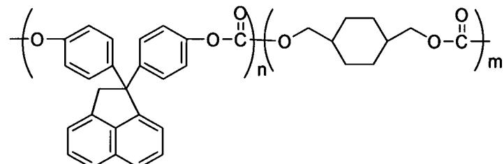
[0103] The optical properties of the obtained resin lens were measured to find that the refractive index was 1.585, the photo-elastic coefficient was  $17 \times 10^{-12}$  m<sup>2</sup>/N and the birefringence was 20 nm. It was confirmed that the lens had a very small birefringence and no substantial optical distortion. The total transmittance was measured to be 89%.
