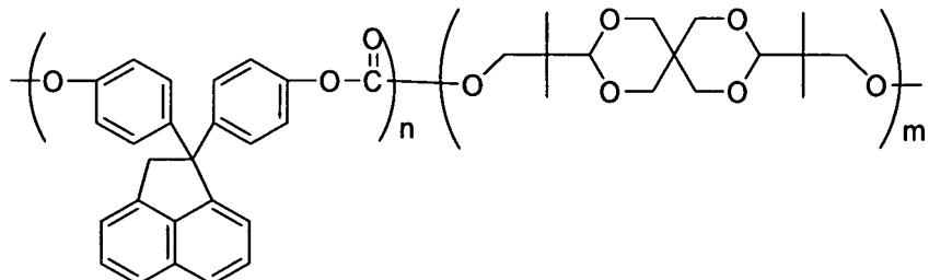
[0105] The optical properties of the obtained resin lens were measured to find that the refractive index was 1.575, the photo-elastic coefficient was  $25 \times 10^{-12} \text{ m}^2/\text{N}$  and the birefringence was 23 nm. It was confirmed that the lens had a very small birefringence and no substantial optical distortion. The total transmittance was measured to be 89%.
