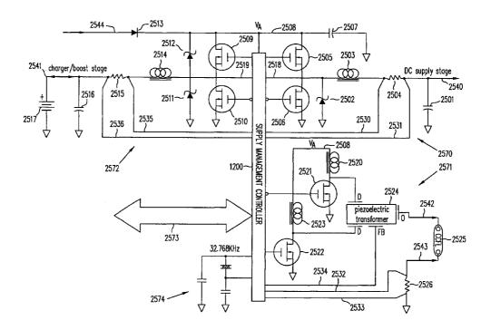
(57) **Abstract:** A control system and method for simultaneously regulating the operation of a plurality of different types of switching power converters. The system utilizes in regulating the power converters sampled data and nonlinear feedback control loops.
