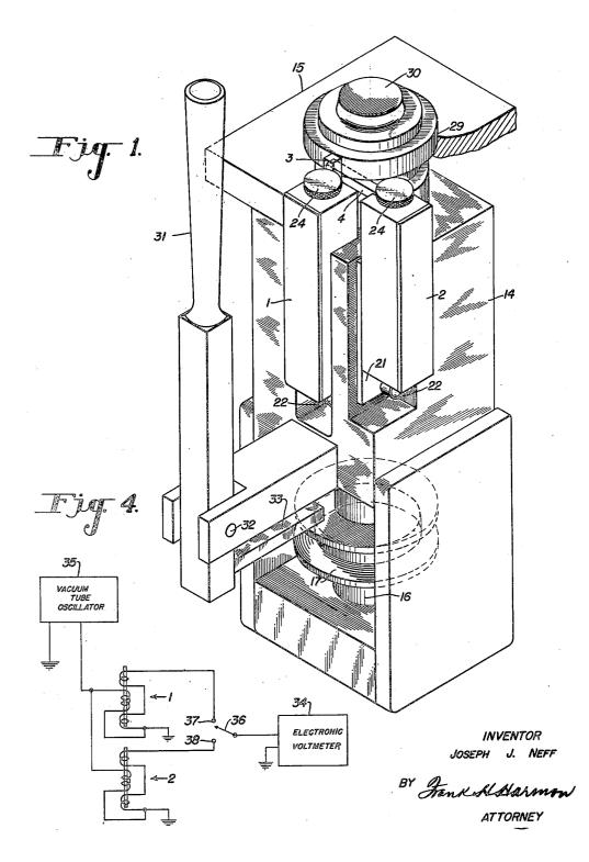
ELECTRONIC CONCENTRICITY AND GROOVE PARALLEL GAUGE
