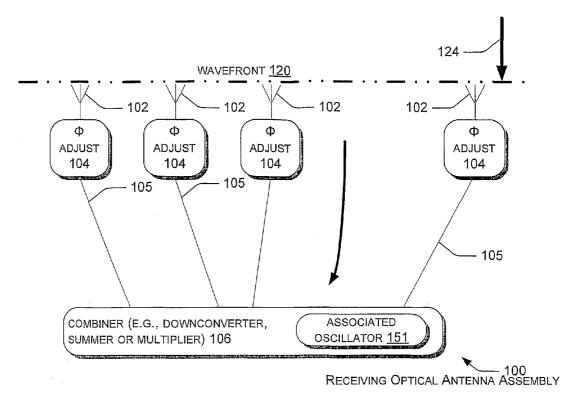
(57) Abstract: An optical antenna assembly including multiple optical antenna elements (102), each of the optical antenna elements are arranged in a regular pattern and carried by a supporting body (202). The regular pattern of the plurality of optical antenna elements is nonuniform. Certain ones of the optical antenna elements are configured to respond to the one or more waves of light.
