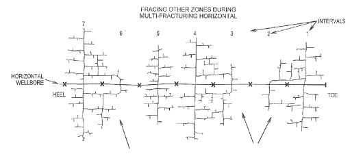
FRAC FLUID WENT INTO OTHER INTERVALS SECTIONS OF RESERVOIR WITHOUT COMPLEX MULTIPLE FRACTURES
