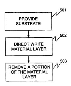
(57) Abstract: A method for fabricating an electronic device comprises providing a substrate (501), direct writing a functional material by a thermal spray on the substrate (502) and removing a portion of the function material to form the electronic or sensory device (503).
