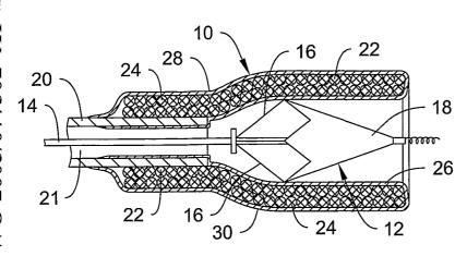
(57) Abstract: A sheath (10) putting an elongate shaft (20) proximate at a distal end and a lumen therethrough. A coil assembly including a first coil (22) defining a lumen. The first coil being wound in a first direction and a second coil (24) wound in a second direction. The second coil being disposed around the first coil. The coil assembly can be attached to the distal end of the shaft and the lumen of the shaft can be in fluid communication with the lumen of the first coil.
