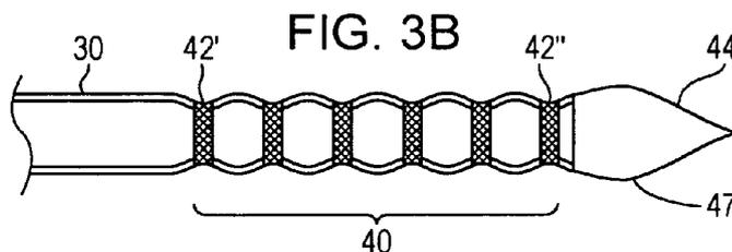
(57) Abstract: An optical fiber diffusion system and a method of manufacturing an optical fiber diffusion device that has a precisely-controlled emission region are disclosed. An optical fiber diffusion device is produced by subjecting a light emission region of an optical fiber to a series of controlled cycles of stress, heating, elongation and cooling, resulting in a pattern of deformation and modification of the fiber and cladding.
