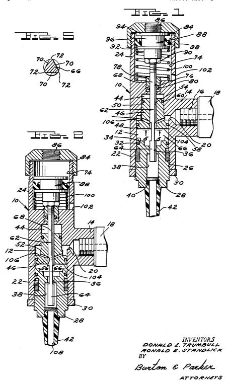
MATERIAL DISPENSING DEVICE INCLUDING A METERING CHAMBER
