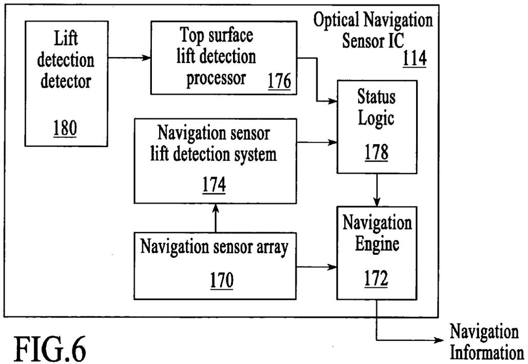
**LIFT DETECTION ADAPTED FOR NAVIGATION ON A TRANSPARENT STRUCTURE**
