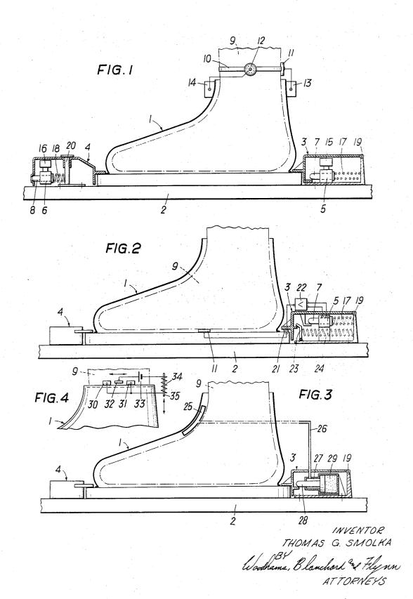
The invention relates to a safety ski binding which releases the ski boot upon occurrence of an overload.
