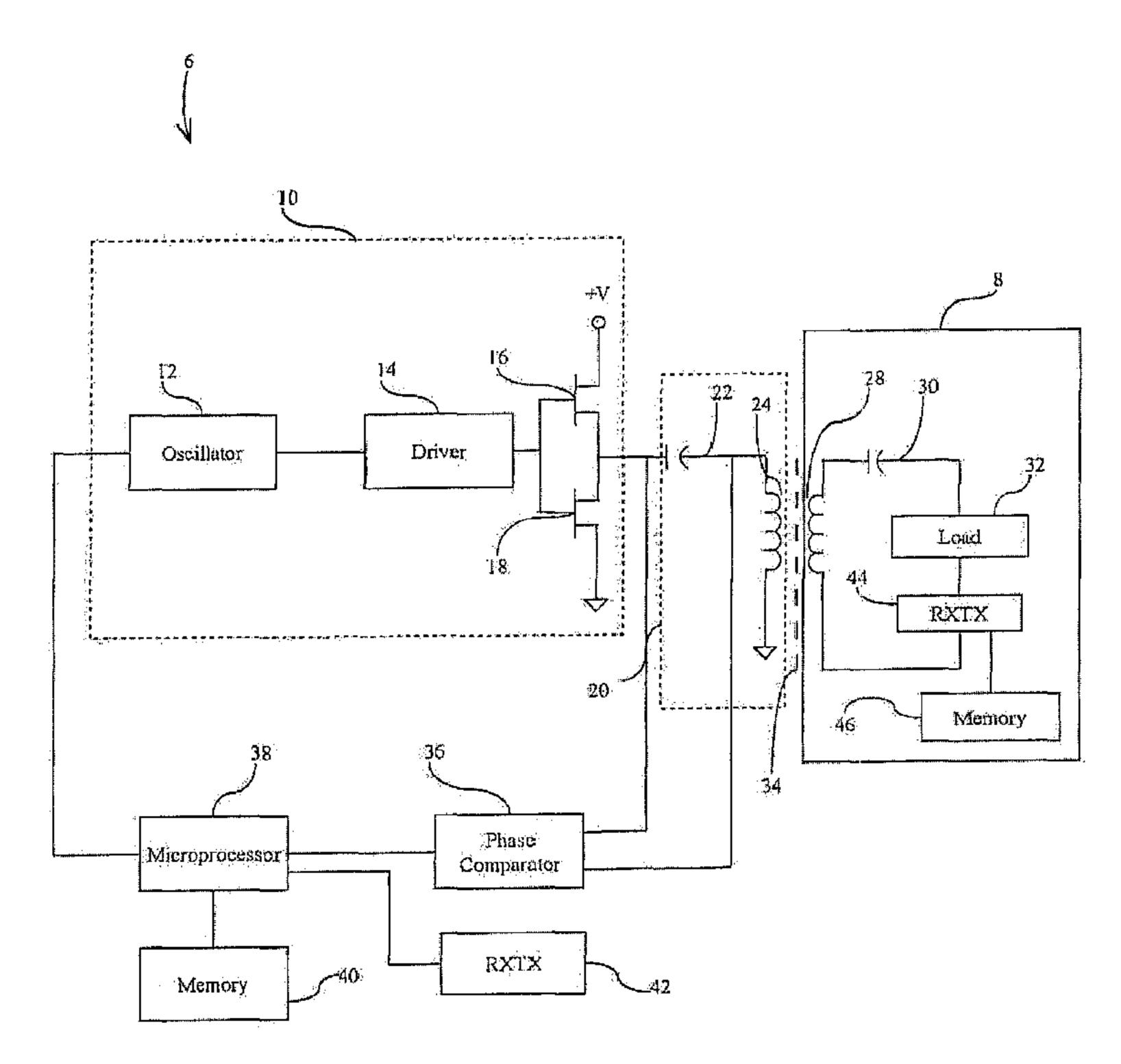
(57) Abstract: A power supply for inductively powering a remote device has an inverter operating at an operating frequency and a primary coil, A phase comparator compares the phase of the voltage or current delivered by the power supply. If the phase relationship detected by the comparator is unacceptable, the inverter is disabled. After a period of time, the inverter is re-enabled, and the phase relationship is again determined.
