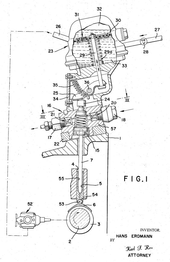
HYDRAULIC PUMP ARRANGEMENT FOR INTERNAL-COMBUSTION ENGINE
