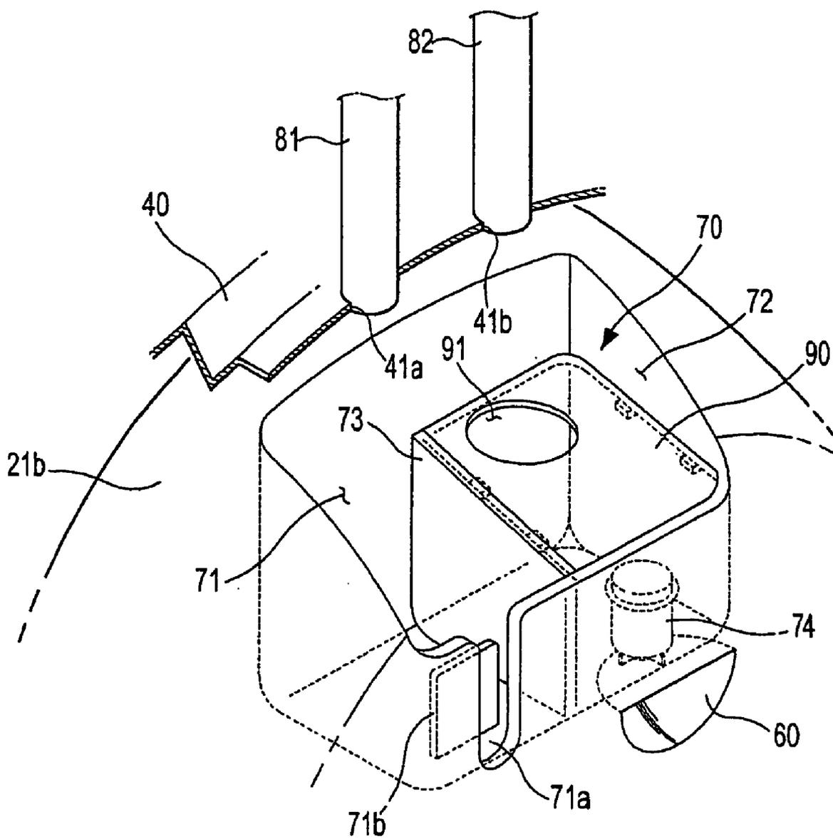
**DRUM WASHING MACHINE WITH DETERGENT SUPPLY DEVICE**
