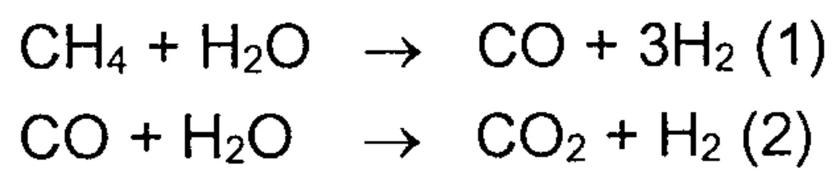
25 The first reaction is strongly endothermic and can directly consume the heat liberated by the electrochemical reaction. This reaction is a catalytic reaction which requires a reforming catalyst (e.g. an Ni catalyst), and it is possible to utilize natural gas (optionally also methane, petroleum gas, naphtha, heavy oil or crude oil) as starting material for operation of the fuel cell.
