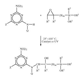
**[0038]** It should be understood that there can be reaction where the hydrogen on each Q reacts with the epoxy, thus allowing the addition of up to 6 epoxy silane units per melamine unit.
