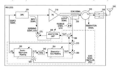
digital pre-distortion adaptation unit configured to determine the distortion control value based on an output signal from the echo signal canceller.
