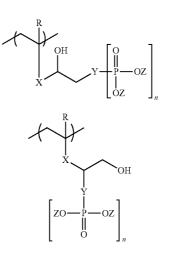
the polymers having a molecular weight of from 800 to 30,000 g/mol, wherein R, X, Y, Z and n are defined as in claim 1.
