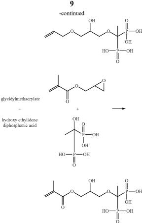
Any such reaction will result in a mixture of compounds of formulae (1a) and (1b).
